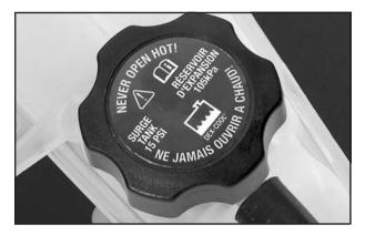
Park the vehicle on a level surface. You can remove the coolant surge tank pressure cap when the cooling system, including the coolant surge tank pressure cap and upper radiator hose, is no longer hot. Turn the pressure cap slowly counterclockwise (left) about one full turn. If you hear a hiss, wait for that to stop. A hiss means there is still some pressure left.
